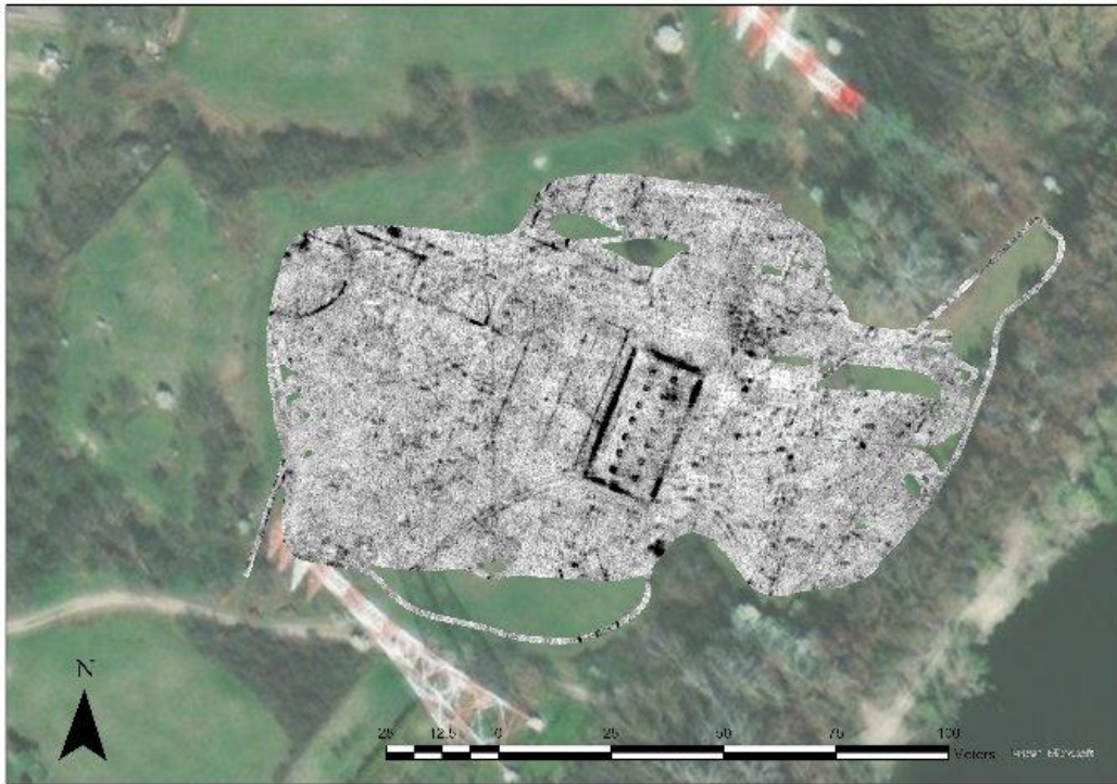
Figure 31: Example of a ground-penetrating radar image. Here you can see details of the interior buildings of the Százhalombatta/Matrica fort (Hungary). Most clearly visible is a warehouse (horreum), surrounded by troop quarters (© LBI ArchPro).
