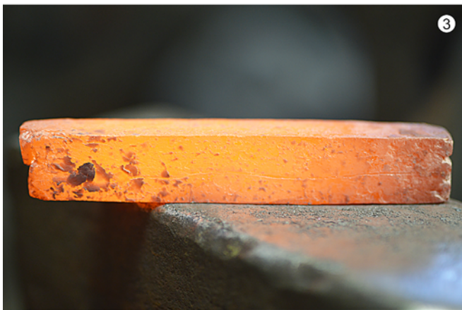
Fig. 7. 1 – Faggoting the rod using forge welding; 2 – welding on the fallen-off parts of the faggot using disodium tetraborate octahydrate (borax); 3 – final prismatic semi-product of a rectangular section with visible traces of faggoting in the form of surface lines. Photo by K. Suchánková.
