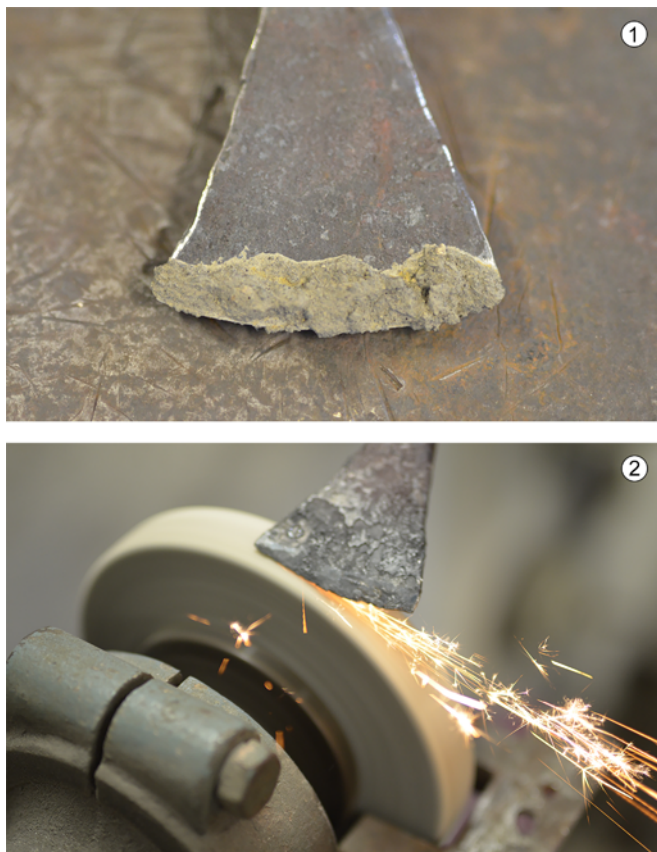
Fig. 5. 1 – The cutting edge covered with the cementing mixture; 2 – spark test on a rotary grindstone indicating how successful the carburisation of the edge was. Photo by M. Hlavica.
