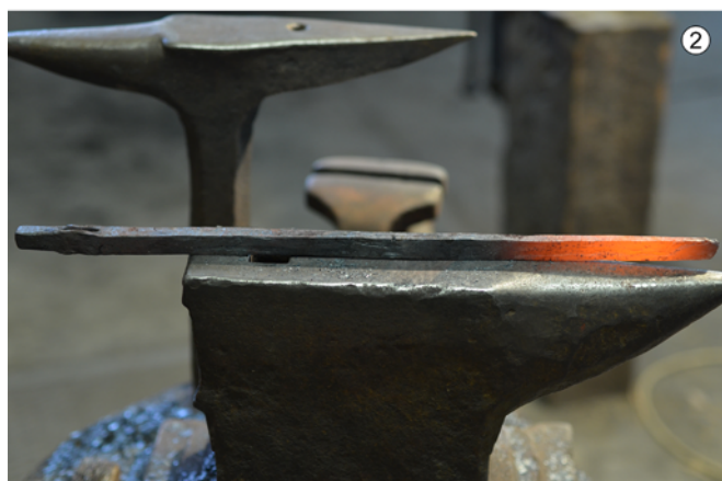
Fig. 6. 1 – Forging down the axe-shaped bar stylized "cutting edge"; 2 – the axe-shaped bar reformed into the shape of a rod of an uneven thickness. Photo by K. Suchánková.
