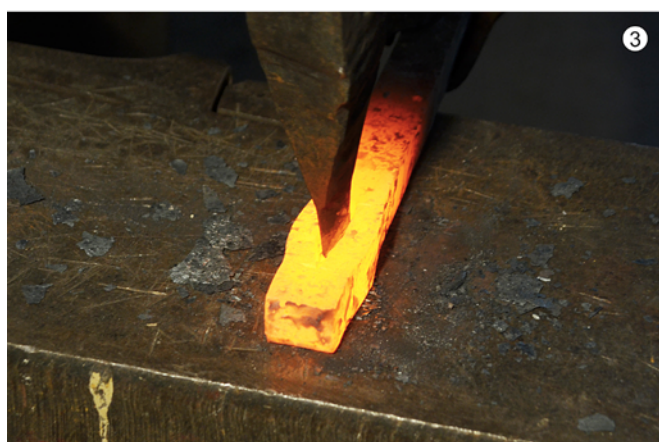
Fig. 3. 1 – A quarter of a non-carburised iron bloom used in the production of replica No. 1; 2 – prismatic semi-product with a square section, the result of the working of the iron bloom, used further in the forging of replica No. 1; 3 – punching the axe eye using a punch with a lenticular section. Photo by K. Suchánková.
