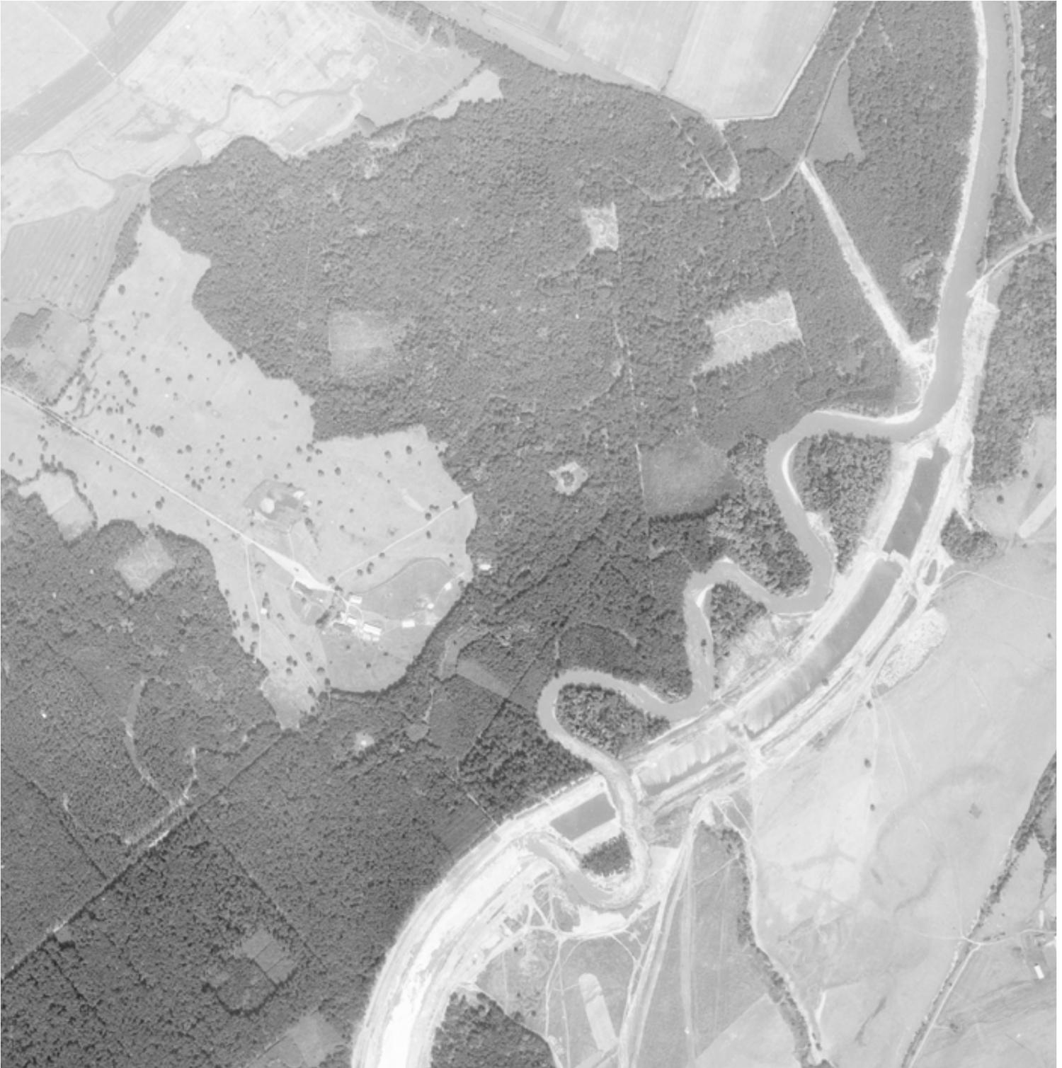
Fig. 39 Aerial photograph from 1970 shows the stream regulation of the hitherto meandering course of the River Morava. This construction ended regular floods and improved conditions for excavation.
